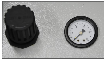
Pressure regulator and gauge for the correct blasting pressure
